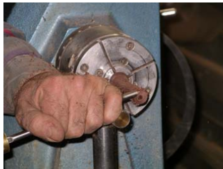
The finial is now reversed in the chuck to refine the shape and cut the thin part to size.
