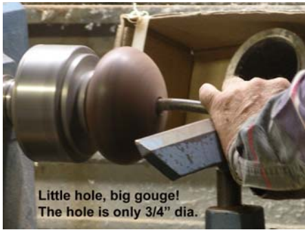
Here you can see the blank for the finial ready to take on it's shape. Note the single round tool rest. Thomas likes this for fine cuts as the tool slides more evenly across the rest.
