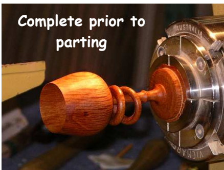
Under cutting the ring w/ skew
