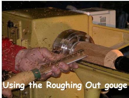
Shaping w/ Spindle Gouge
