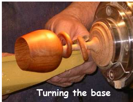
Under cutting the ring w/ skew
