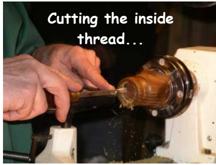
Starting the bottom, note the "sizing shoulder"
