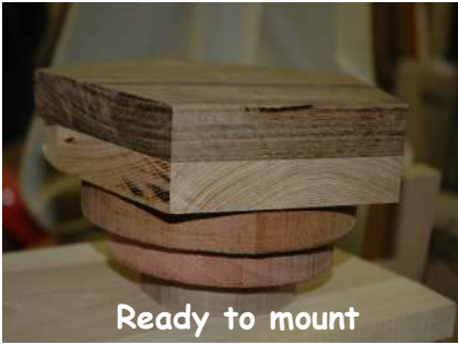
Mounted on a screw chuck— ready to begin shaping process
