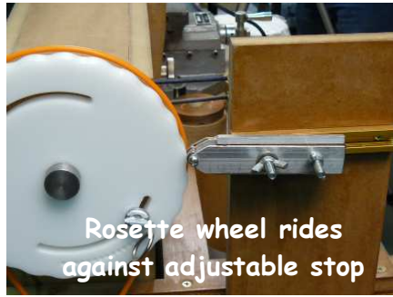
Cross sled holds cutter on the Rose engine lathe
