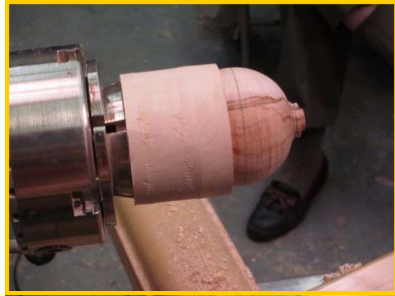
Sphere mounted in jam chuck
