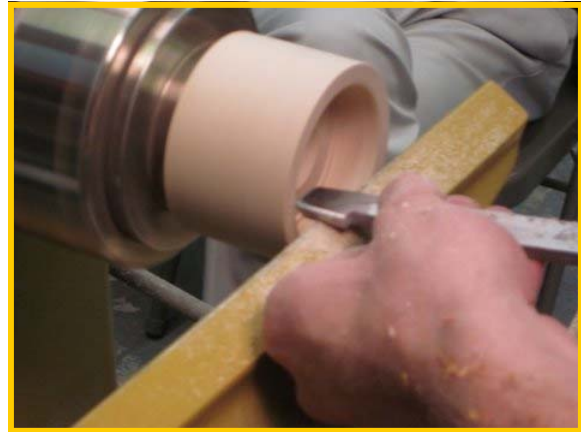
Making the opening larger to accept the blank
