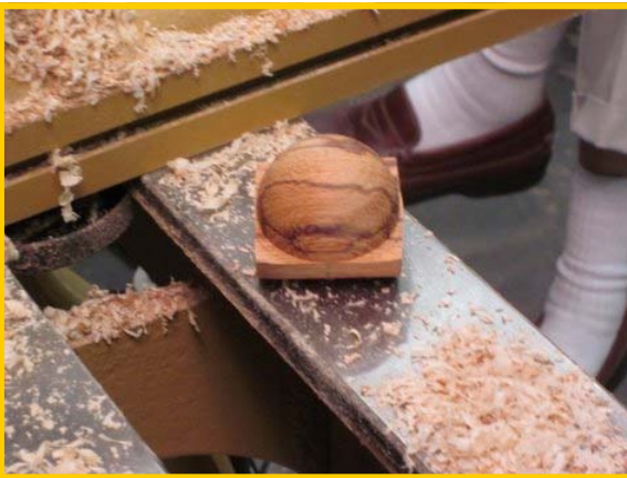
Blank removed from first jam chuck, ready to be reversed in smaller jam chuck
