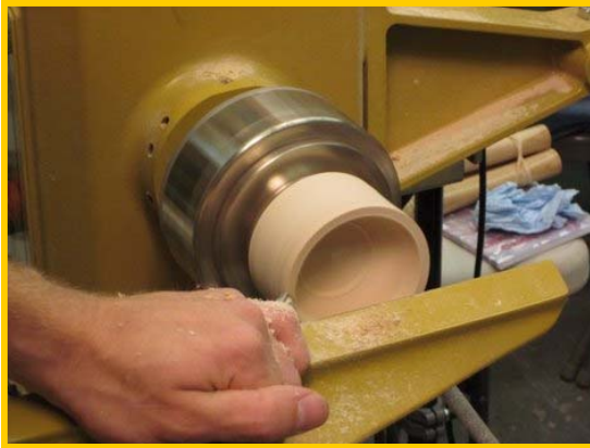
Shortening the chuck to get a smaller diameter
