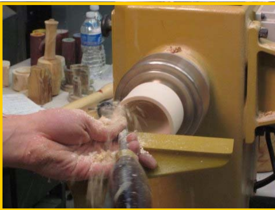
Jam chuck mounted and making it fit the sphere
