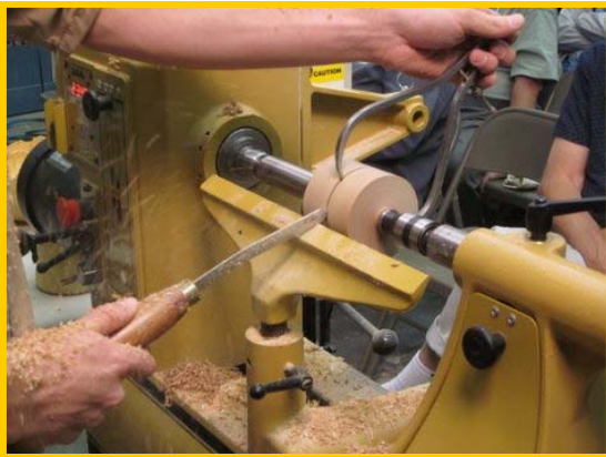
Setting the diameter of the sphere with a caliper measurement
