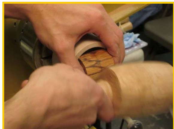
Making sure the blank is secure
