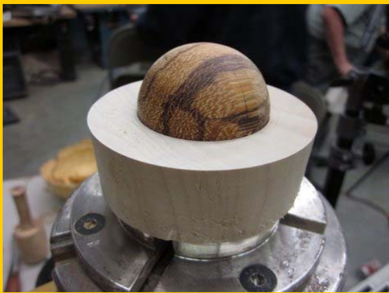
View of finished sphere before removing it from the jam chuck
