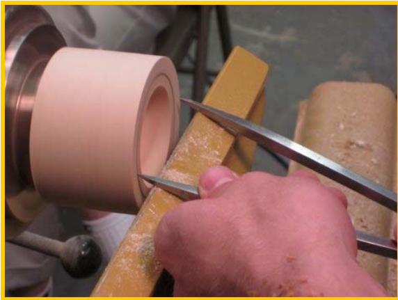
Measuring the jam chuck opening
