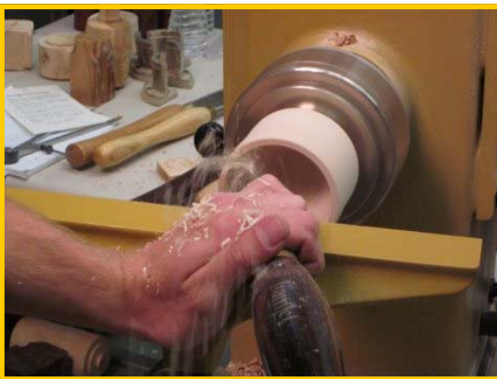
Making the chuck bigger to accept the sphere when he turns it
