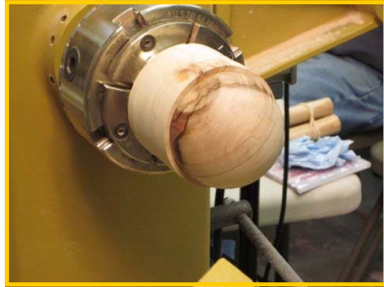
Making the chuck bigger to accept the sphere when he turns it
