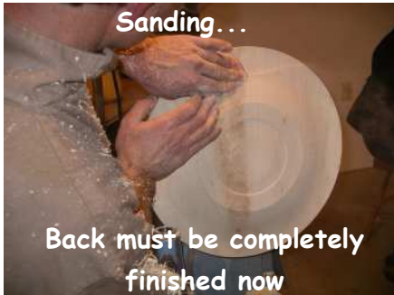
Platter blank mounted, Mike develops shape of back
