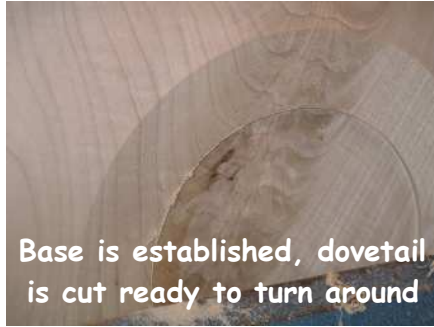
Platter blank mounted, Mike develops shape of back
