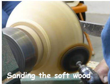
Showing the unstable wood, the ring holds it together
