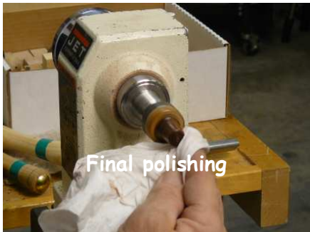
Mounted on shop-made mandrel to finish dome
