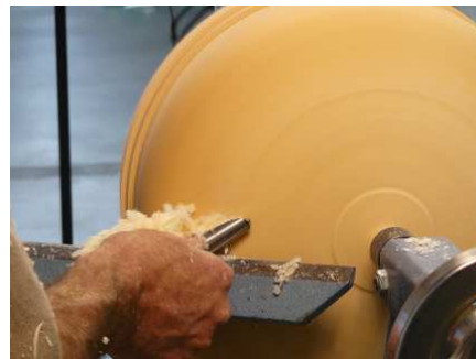
Shear scraping refines contour
