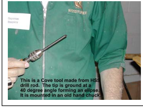
The Cove tool is used to make small coves on edges and areas that are very delicate. The pattern came from the AAW magazine in the spring of this year.
