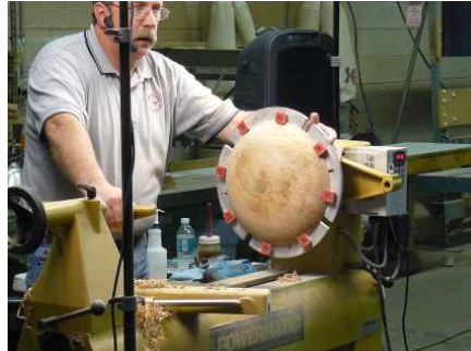
Mounted on Cole Jaws
