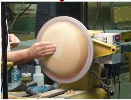
Hand sanding the footless
