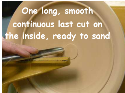
Rim is finished, stepping down to remove waste from the interior
