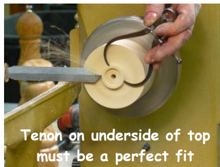
Top is now mounted in chuck, ready to drill and form tenon
