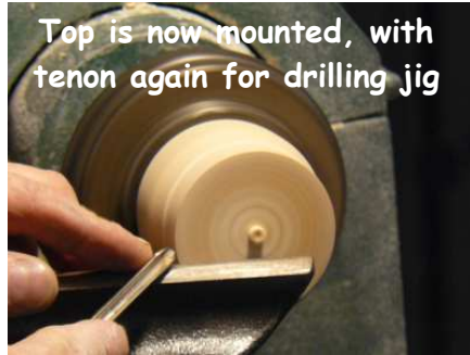
Tenon is for drilling jig, note holes for pillars
