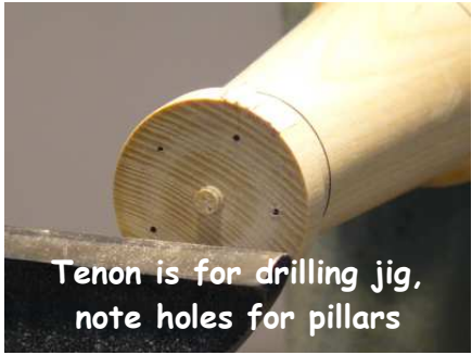
Top is now mounted, with tenon again for drilling jig
