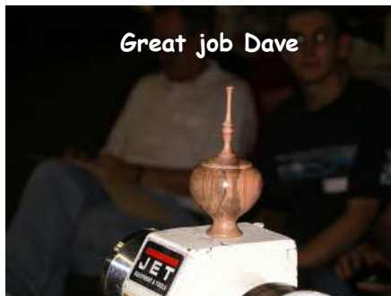
Nylon jaws holding the base to finish the bottom
