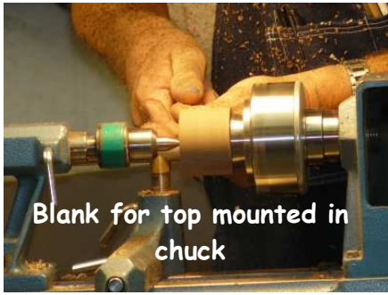
Top where it will join to body cut concave for a tight fit
