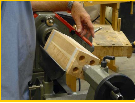
Mounting the blank to make 4 candlesticks
