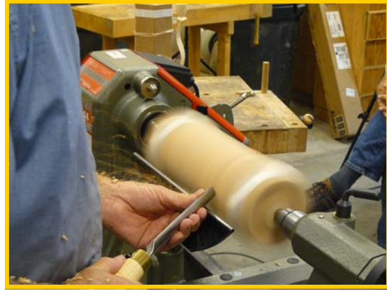
Mounting the blank to make 4 candlesticks
