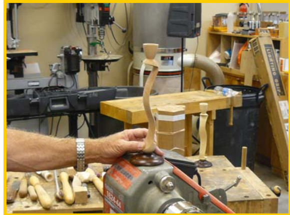
Bottom done and ready to take out of chuck.
