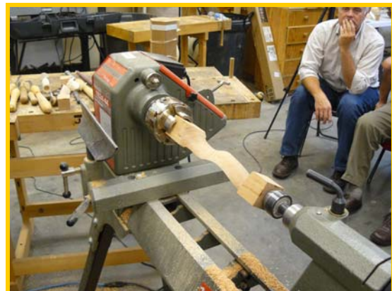
Now mount one candlestick in a 4-jaw chuck with a cone center in the top
