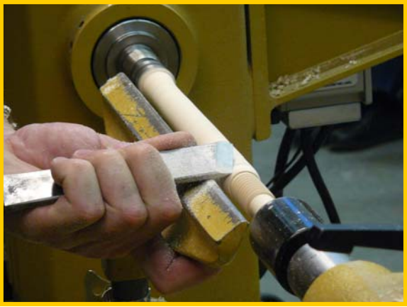
Removing excess wood
