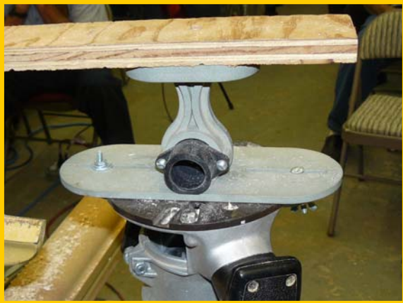
Beall wood threading jig Note: The insert was drilled to the threaded portion to minimize the gap between the threads and handle.
