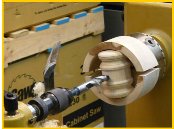
Drill mounted in tailstock, ready to drill
